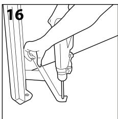
Concrete fix the support legs into the ground as per Fig 10, 11 and 12 (Step 2).
