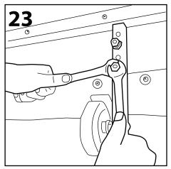
closest to the wheel support bar. Using a second spanner unscrew the outermost nut and remove. Repeat on other wheel support bar fixing point.
