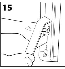
Replace the bolts and washers into the new holes through the the spigot leg. Tighten with 13mm spanner/socket.
