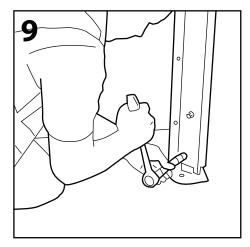
Replace the bolts and washers into the new holes within the spigot leg and tighten with spanner/socket. Repeat Figs 7 -9 on the other legs that need adjusting.
