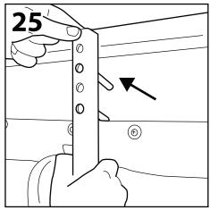
Lift the wheel support bar off the bolts, ensuring that the door is still supported.
