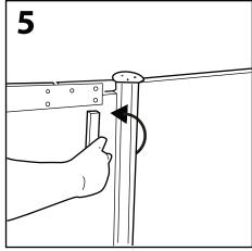
After replacing the wheeled bin, remove the door stay catch by pushing upwards anticlockwise so that is positioned vertically.
