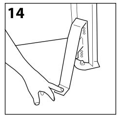
Place the support leg (B) up against the inside of the extrusion so that the leg protrudes outwards support leg, extrusion and into and stands on the ground. If the spigot legs have been adjusted there are several pre-drilled holes in the support leg to accommodate this adjustment.
