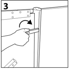
To ensure that the door remains open whilst removing the wheeled bin, turn the door stay catch clockwise so that it is positioned horizontally.
