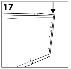
If the door is not level, as seen above, the door wheel can be adjusted.
