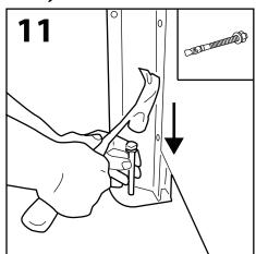
The fixing bolts (A) MUST appear as the top of the bolt. Using a hammer, tap fixing bolt through the hole in the spigot leg until it is flush with the spigot plate.
