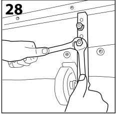
Holding the nut with the 17mm spanner, place the second nut over the bolt and tighten securely with a second spanner. Repeat figs 27 and 28 using other fixings.
