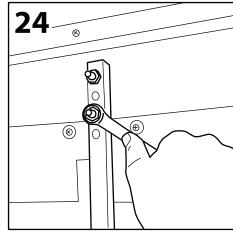
Using 17mm spanner, hold the nut Using 17mm spanner remove the second nut and washer. Repeat on other wheel support bar fixing point.
