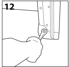
Tighten bolt using 17mm spanner. Repeat Figs 10 - 12 to ground fix the other extrusions.
