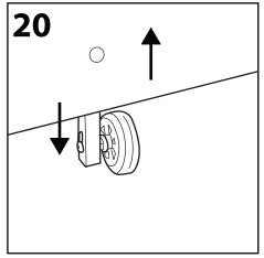
Lift door panel and pull wheel down so that the axle drops down the slot in the wheel support bar (may require two people.)
