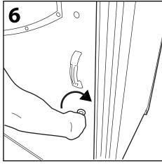
Close the door and insert key into lock. Turn key clockwise to lock door. (Alternatively: Turn twist lock clockwise to lock door.)
