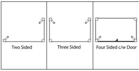
Using a 13mm spanner/socket unscrew the two bolts with washers at the bottom of the outermost extrusions and remove. (see diagrams above showing location of support legs for all screen types) If the spigot legs have been adjusted (Step 1) the panels will need to remain lifted in position so that the support legs go into the correct holes. (may require two people.)
