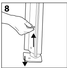
Lift the extrusion upwards and pull the spigot leg down to a more appropriate height ensuring that the screen is now level.
