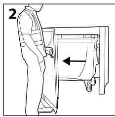
Using handle pull door open to 90 degree position.
