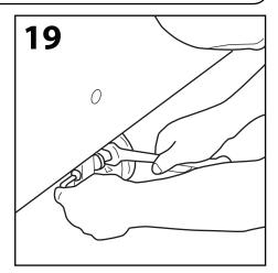
Using 17mm spanner and 6mm allen key, loosen nut on left side of the wheel to free the axle from the wheel support bar.
