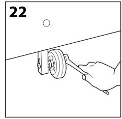
Tighten up nyloc nut (right of wheel) ensuring that wheel can still rotate freely but is secure on the axle.
