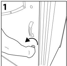
Insert Glasdon Key into lock and turn anticlockwise to unlock the door. (Alternatively: Turn twist lock anticlockwise to unlock door.)
